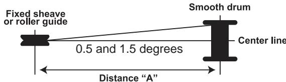
2. Wire rope moves directly to the load. Use tracks or guide rails to prevent sideway movements that can stress and harm the drum flange.
